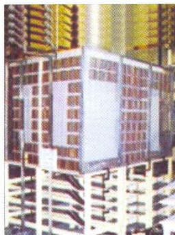
Internal arcing withstand test
