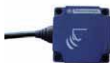
"Bad" part (marking incomplete)
