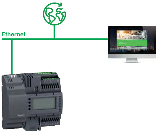
M172 optimized logic controller linked to Ethernet via the TM171AETH or TM171AETHRS485 communication module
