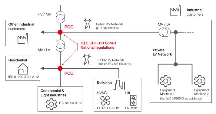
The THD<sub>u</sub> limits are considered at the PCC within the public network (LV or MV) from where the different customers are supplied by the Utility. Limits must be applied at the PCC in order to ensure the Utility (often by duty constraints) supplies the different customers with a good quality of power, i.e. with non distorted voltage.
