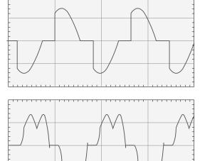
When dealing with non linear loads, we should consider the individual current of each non linear device and the combination of currents for all loads, including linear loads.
