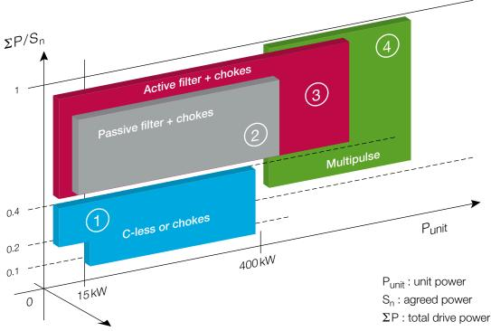
The two considered criteria are the unit power of the installed drives ( $P_{unit}$ ), and the ratio of the total power of drives ( $\Sigma P$ ) related to the agreed power of the installation ( $S_n$ ).
