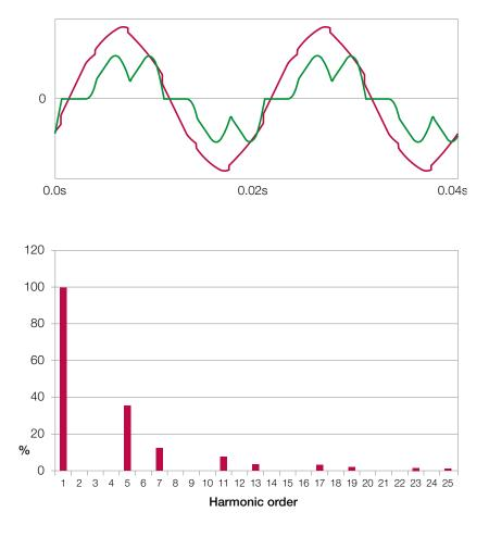
The current distortion can be reduced by implementation of harmonic mitigation. As an example, the improvement provided by a 12-pulse arrangement is presented on the opposite figure. THD<sub>i</sub> is reduced from 40 to 11%
