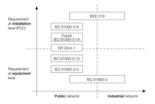
It should be noted that too stringent harmonic emission limits could become very expensive. That's why a careful application of standards should be performed. The following diagram is proposed for clarification.
