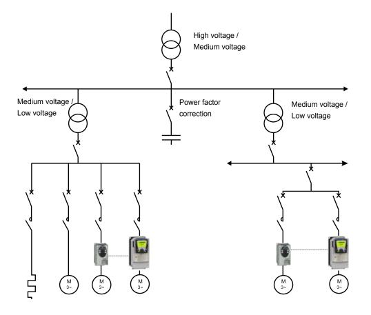
For a big plant, the incoming power from the public supply system is provided through a high voltage step down transformer which is installed at the factory level.
